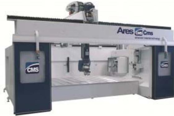
The term “5-axis” refers to the ability of a CNC machine to move a part on five different axes at the same time, allowing the cutting tool to approach the part from all directions for versatile cutting of complicated work piece without any compromise in rigidity or stability.
